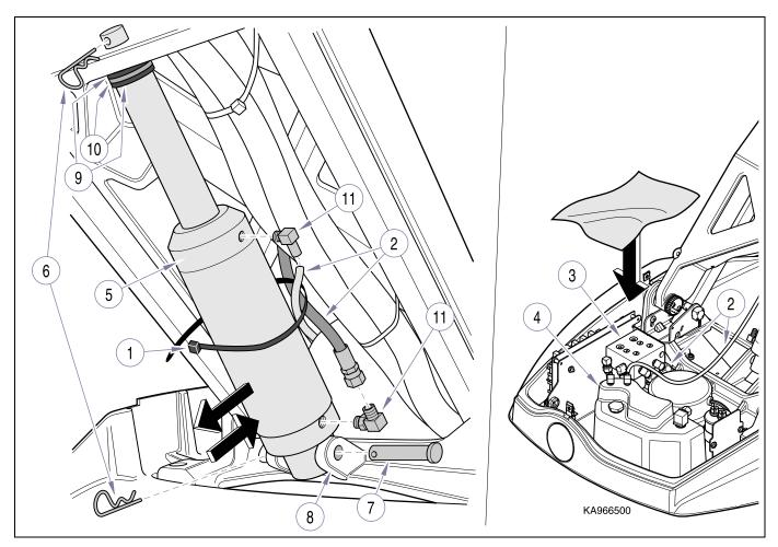
Figure 4-9. Hydraulic Base Cylinder
