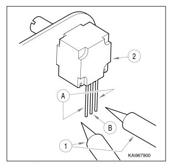
Figure 2-8. Testing Potentiometer.
