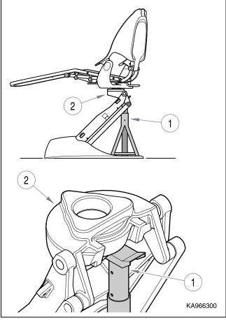
Figure 4-7. Hydraulic Base Cylinder
