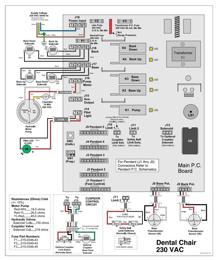
Fig. 5-8. 230 VAC PC Board and Related Circuitry (Used on Serial Numbers V1969965 to present)
