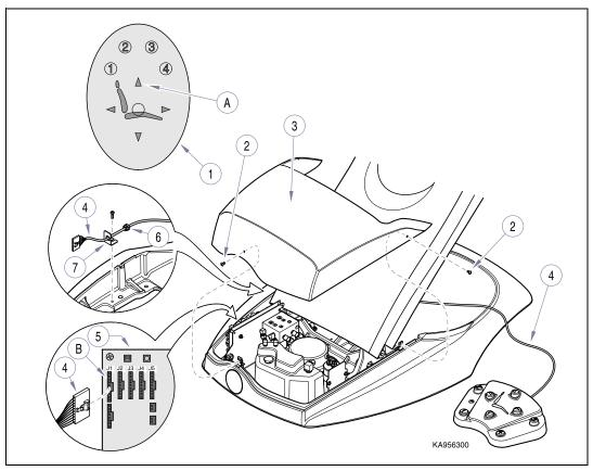
Figure 4-26. Foot Switch Control
