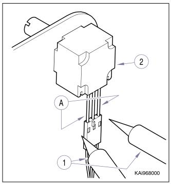
Figure 2-9. Testing Potentiometers
