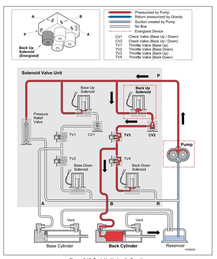
Figure 5-15. Back Up Hydraulic Function
