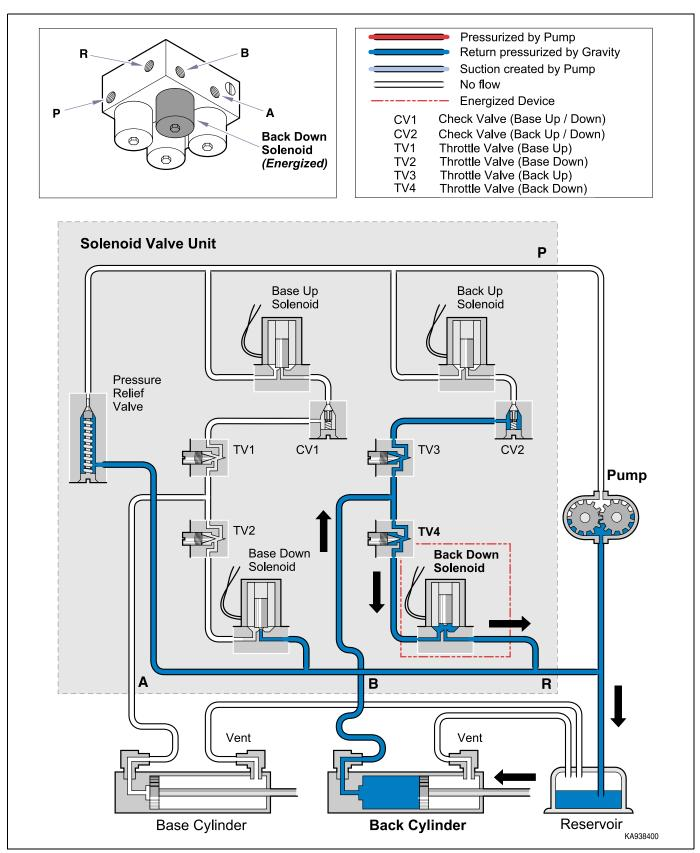
Figure 5-16. Back Down Hydraulic Function
