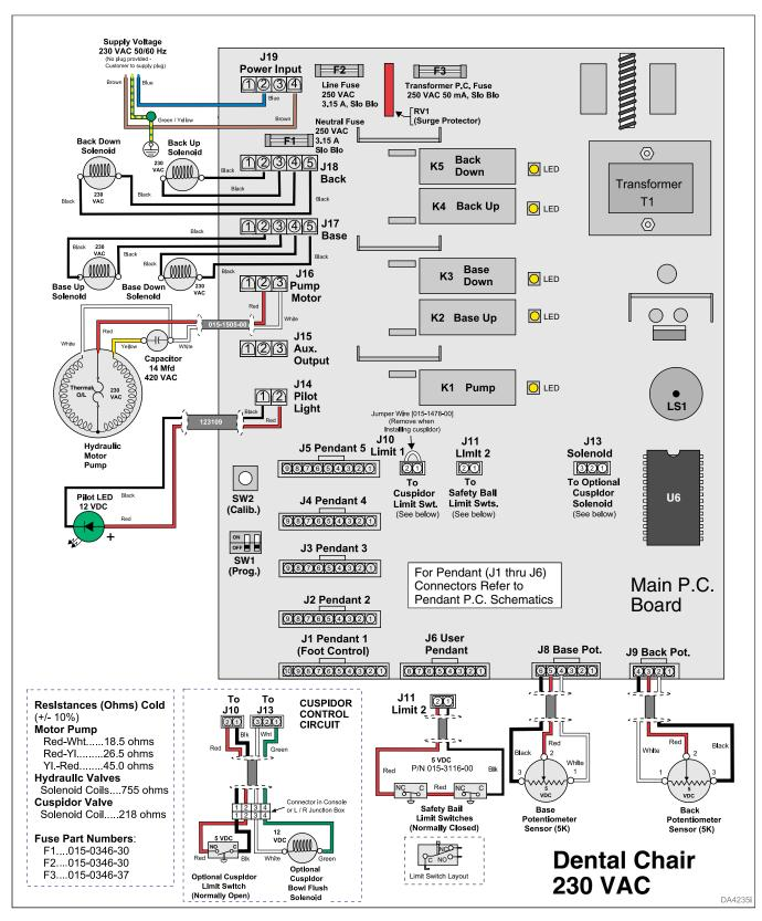
Fig. 5-7. 230 VAC PC Board and Related Circuitry (Used on Serial Numbers V1314210 to V1969964)
