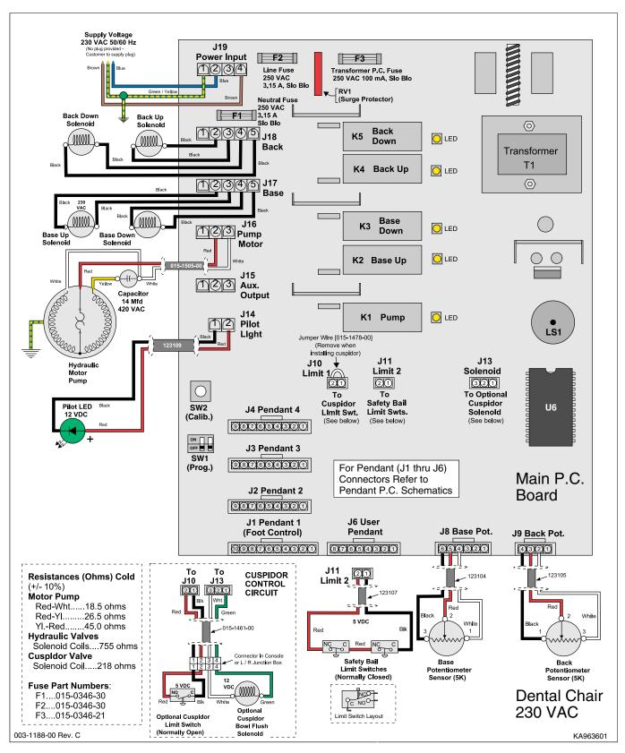
Fig. 5-5. 230 VAC PC Board and Related Circuitry (Used on Serial Numbers NZ1000 thru NZ1019)
