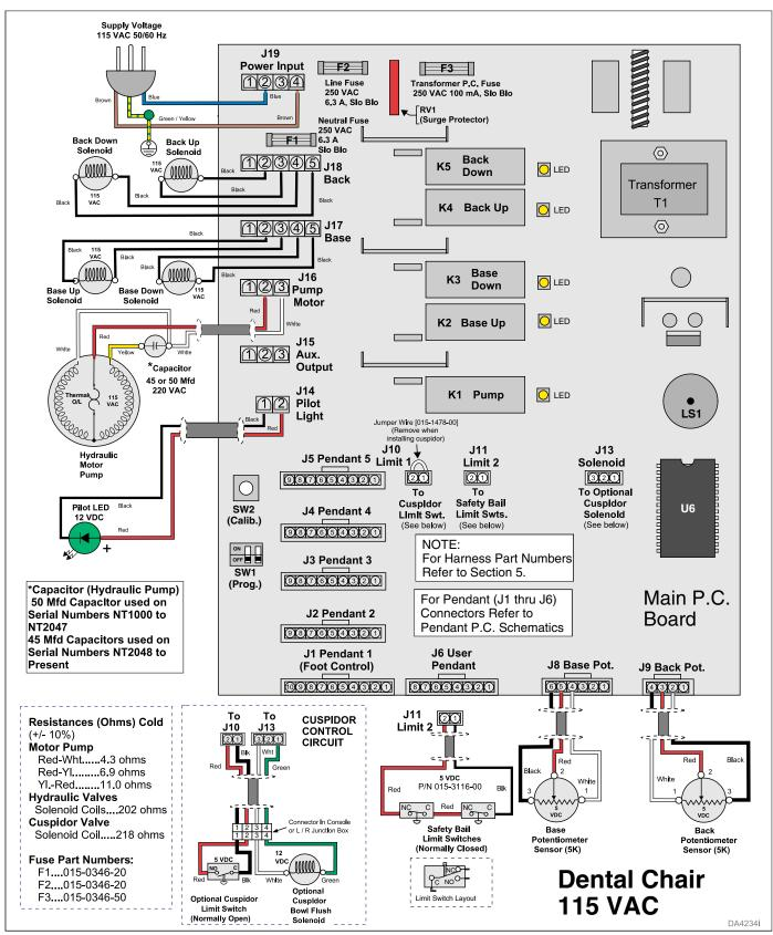
Fig. 5-3. 115 VAC PC Board and Related Circuitr y (Used on Serial Numbers V1314210 to V1969964)
