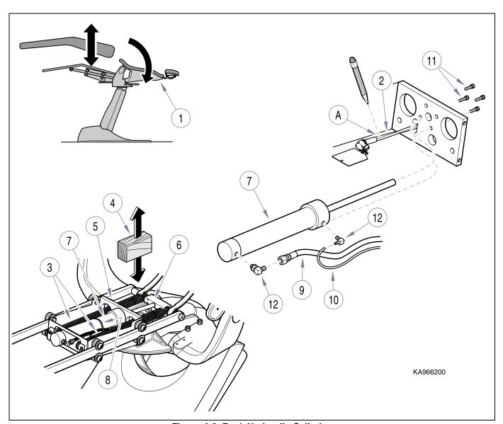
Figure 4-6. Back Hydraulic Cylinder
