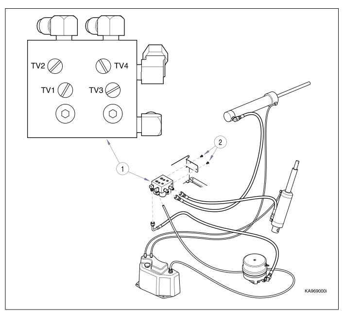
Figure 4-16. Hydraulic Solenoid Valve Assembly.
