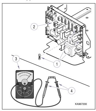
Figure 4-18. Fuse (P.C. Board)
