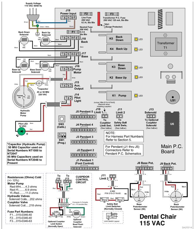
Figure 1-4. Main P.C. Board and Related Components (Current Production)
