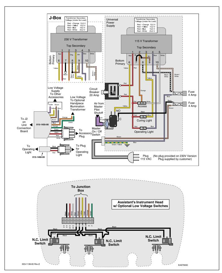
Figure 5-11. J-Box and Assistant's Instrument Head Diagram (115 or 230 VAC)
