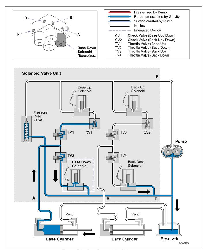
Figure 5-14. Base Down Hydraulic Function
