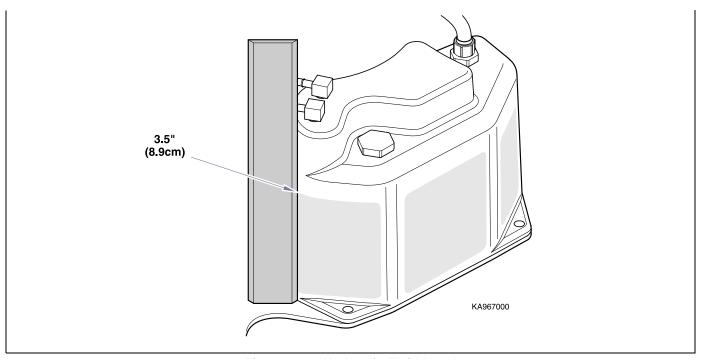
Figure 4-13. Hydraulic Fluid Level
