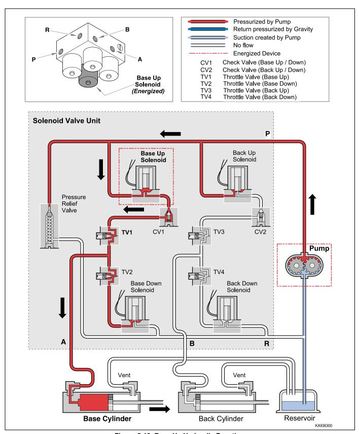
Figure 5-13. Base Up Hydraulic Function
