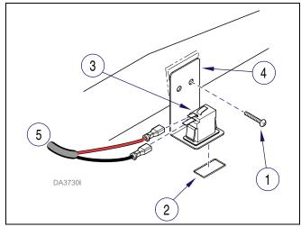
Figure 4-24. Safety Bail Limit Switch.
