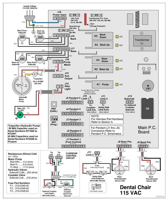
Fig. 5-4. 115 VAC PC Board and Related Circuitry (Used on Serial Numbers V1969965 to present)
