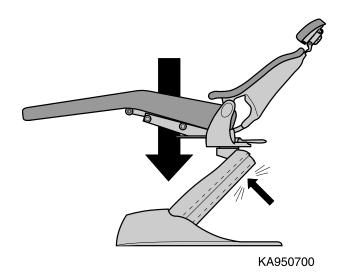
Figure 2-5. Safety Bail Limit Switches.
