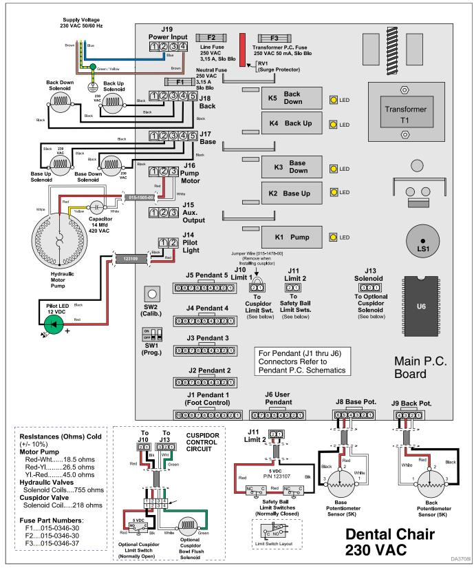
Fig. 5-6. 230 VAC PC Board and Related Circuitry (Used on Serial Numbers NZ1020 thru V1314209)
