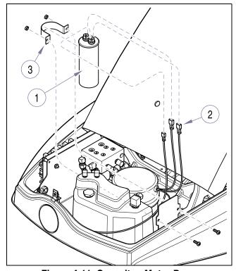
Figure 4-11. Capacitor, Motor Pump
