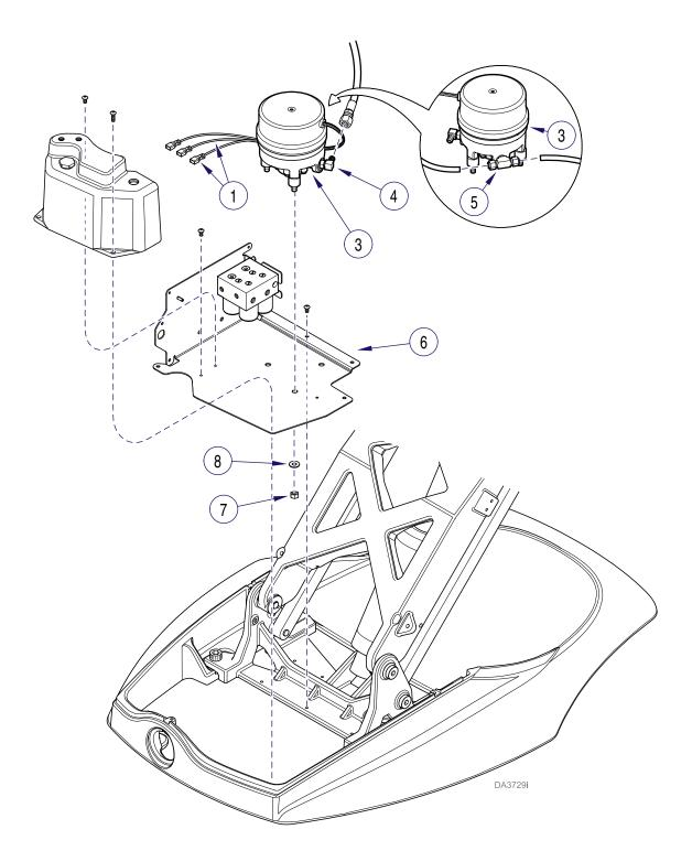
Figure 4-10. Hydraulic Motor Pump
