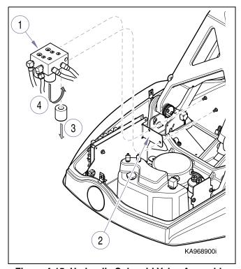
Figure 4-15. Hydraulic Solenoid Valve Assembly.
