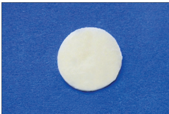
Figure 3. Photograph of a glass ionomer sample. (Photograph courtesy of Peggy Cain, UNMC College of Dentistry Photographer.)
