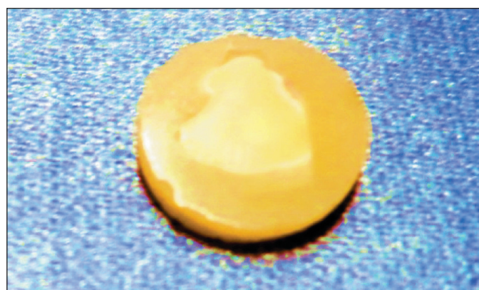
Figure 5. Enamel sample embedded in composite material prior to treatment with an air polishing powder.
