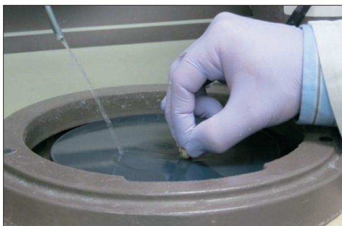
Figure 2. Photograph illustrating the wet polishing of samples to create uniformly smooth surfaces.
